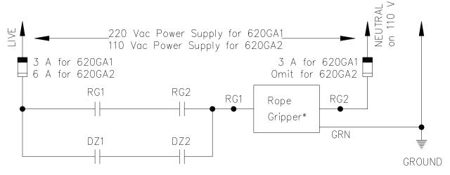
\*See Diagram 4 for Rope Gripper circuits
